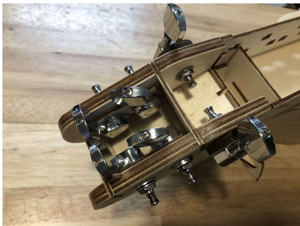
Mount the other tuners, with the wooden spacer on the inside, and an extra washer on the outside. You do not need the little screws that come with the tuners, but if you can find a way feel free to put them in.
