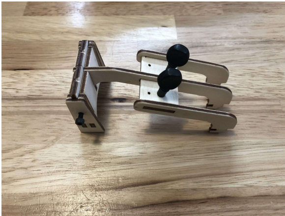
Grooves should be filed into the bridge segments, so that you're sure that the string is touching it at the front.
