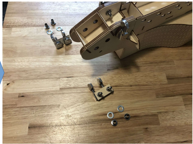
Mount the tuners for the melody strings use part NG-31
