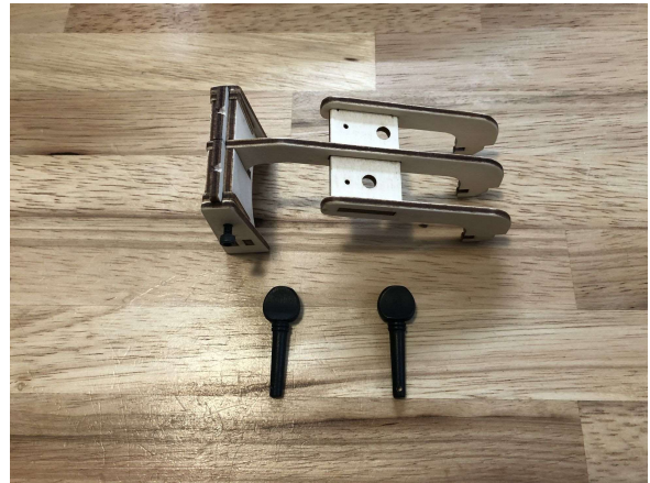
Grooves should be filed into the bridge segments, so that you're sure that the string is touching it at the front.
