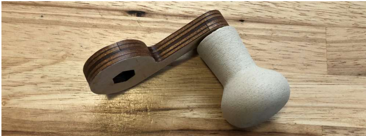
Gently press the knob onto the bearings
