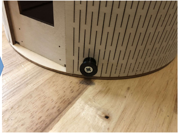
The plate goes on the inside, and is meant to divide the force over a larger area
