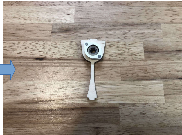
Combine the two plates that will support the front bearing
