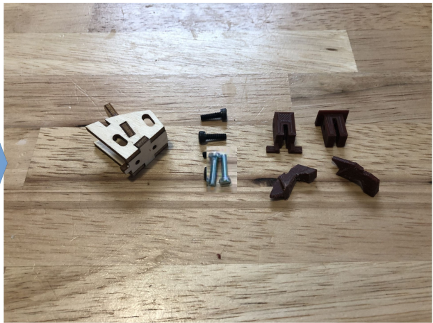
Put the M3 nuts into the buzzing bridge supports use parts NG-4, NG-5, NG-18
