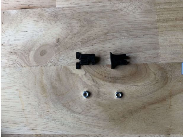
Put the M3 nuts into the buzzing bridge supports use parts NG-4, NG-5, NG-18
