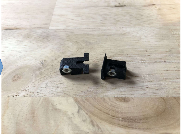
Put the M3 nuts into the buzzing bridge supports use parts NG-4, NG-5, NG-18
