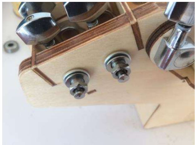
Mount the other tuners, with the wooden spacer on the inside, and an extra washer on the outside. You do not need the little screws that come with the tuners, but if you can find a way feel free to put them in.
