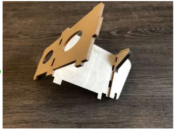
Insert the small plates from the rear
