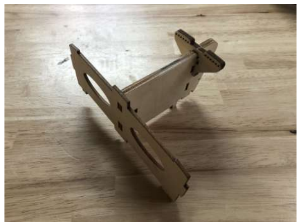
Insert the 6mm plate from the top
