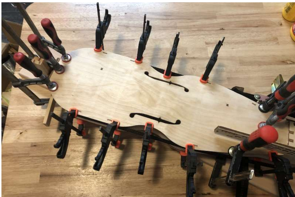
Not all the inner parts will follow the profile of the top plate perfectly, so apply ample glue to make sure everything is attached.
