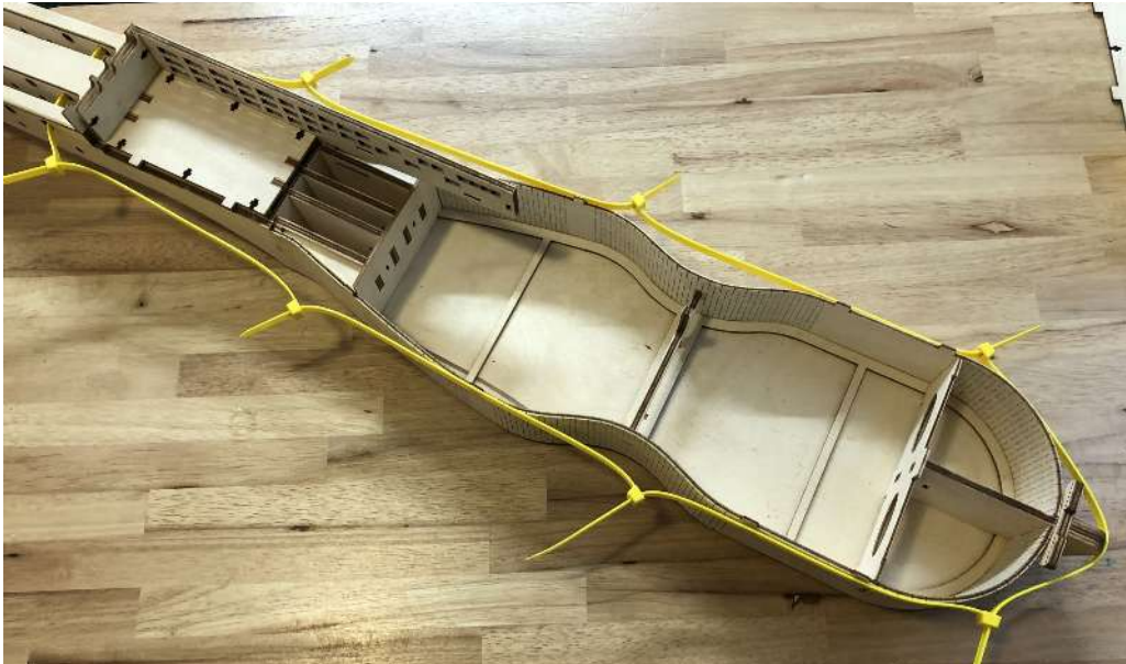
Preparing cable ties to pull the front and back together during gluing
